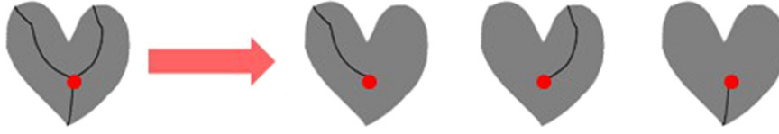
Fig. 3. A junction point and its junction paths.
