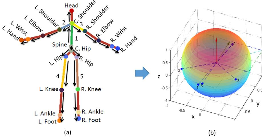
**Fig. 2.** (a) A skeleton and its joints. The C. Hip is the root of the kinematics chains formed by joints (marked by arrows). (b) An illustration for the skeleton feature computation. For better visualization, only 5 joints are shown in the unit sphere.
